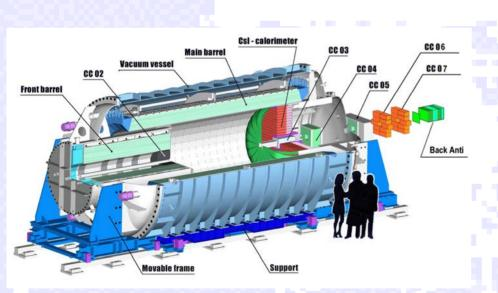
•The original KOPIO concept measures the kaon momentum and photon direction...Good! But costs detector acceptance and requires a large beam to compensate.
