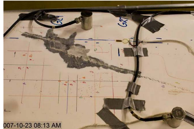
Figure 27: TX-100 high-pressure skin damage area.
