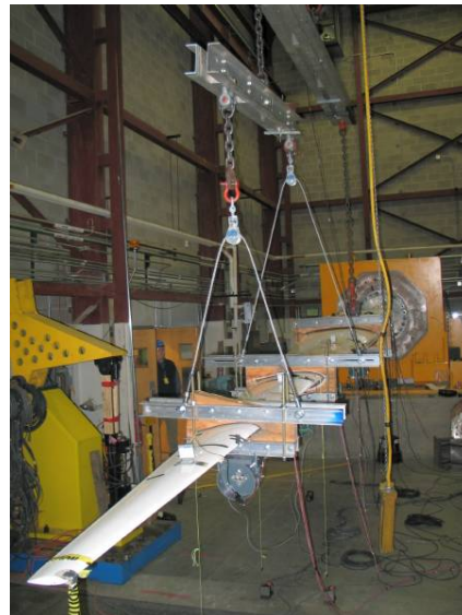
Fig. 13. TX-100 Static Testing
