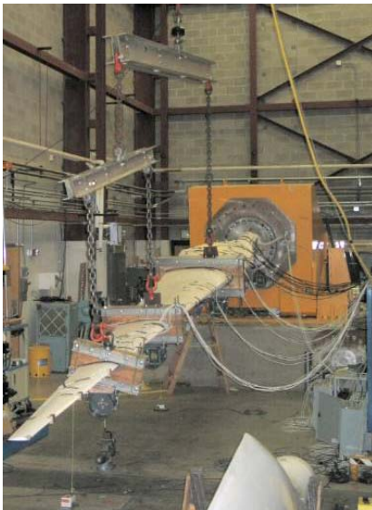
Fig. 12. CX-100 Static Testing
