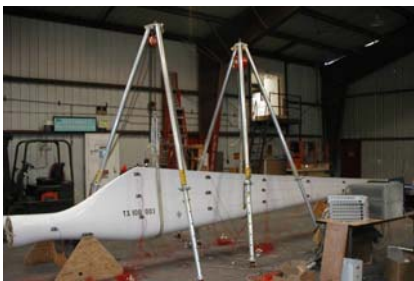
Fig. 9. Modal Test Set-up
