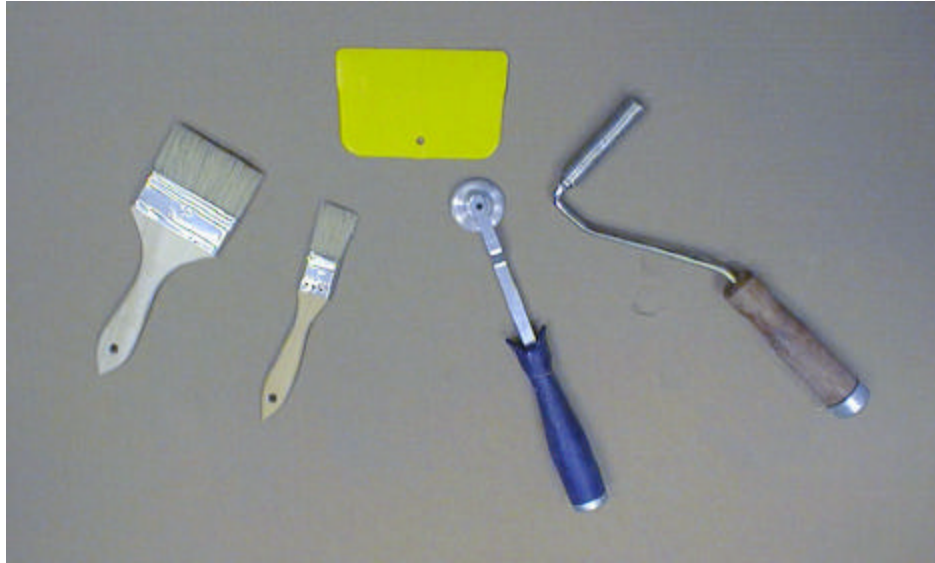
Figure 3: Tools used in hand lay-up.
