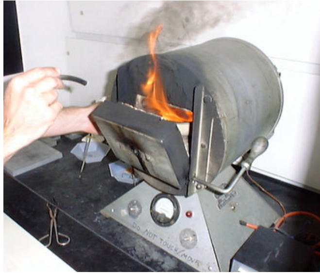
Figure 10: Burn-off test showing combustion products.
