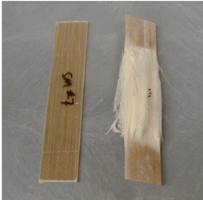
Figure 16: Before and after ultimate tensile strength test of fiberglass.
