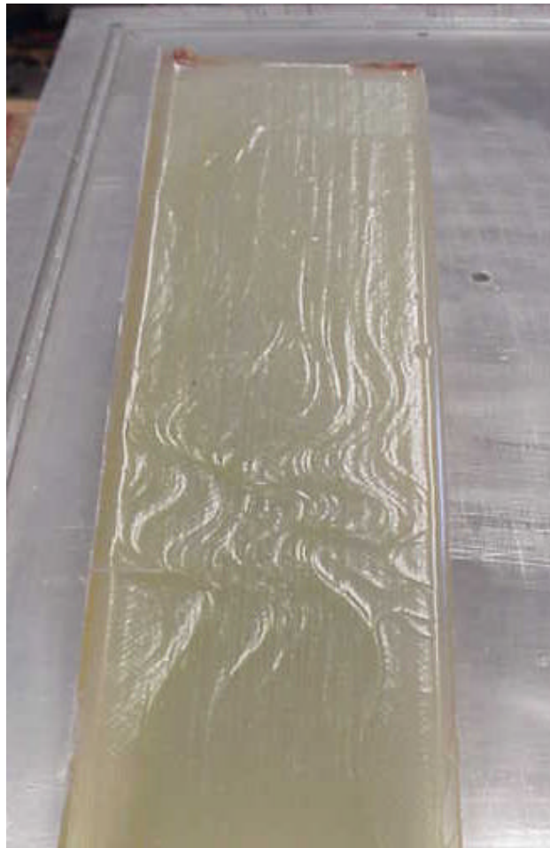
Figure 37: Catastrophic fiber wash on top layer of injection port end of 244 cm plate.
