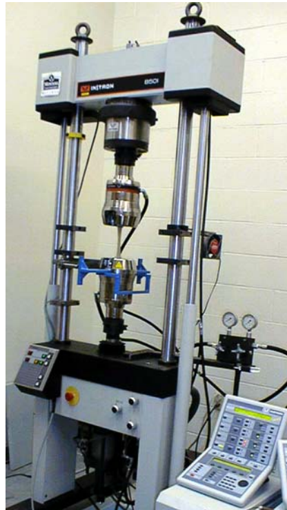
Figure 16. Instron 8501 servo-hydraulic testing machine at MSU
