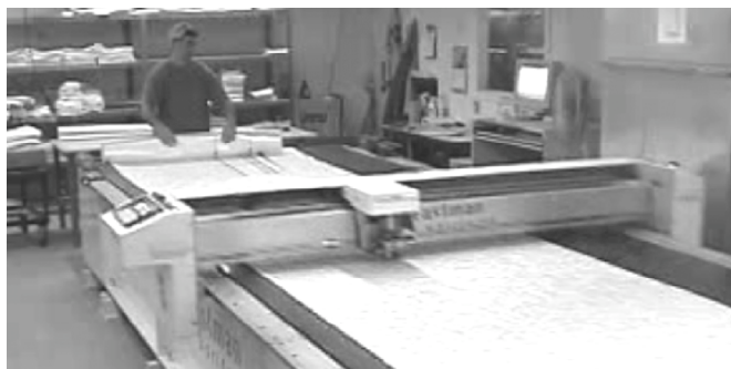
Figure 2.9 Automated Fabric Marking and Cutting
