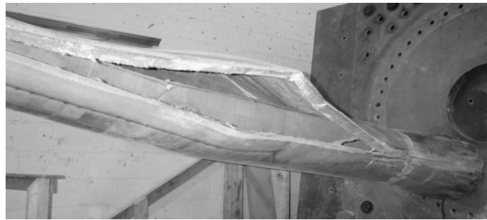
Figure 2.24 NPS-100 Static Failure on 15 February 2002 Test
