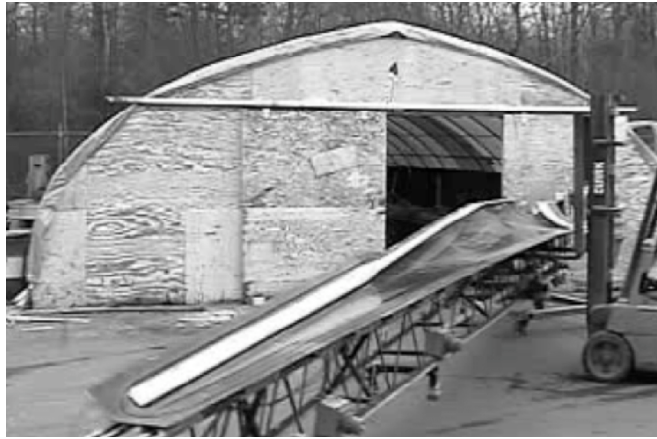
Figure 2.8 Movement of Blade Skin Molds Into the Structure
