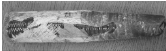
Figure 3.10 Failed M30 Stud From Specimen #1
