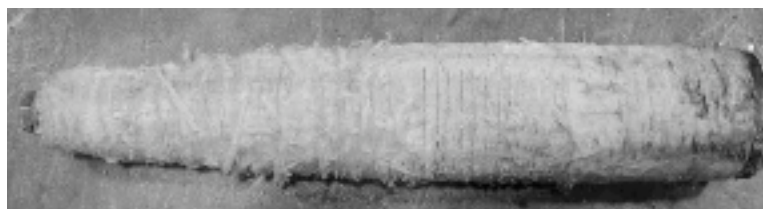
Figure 3.11 Failed M30 Stud From Specimen #6
