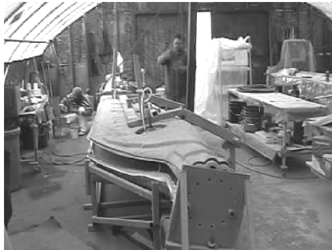
Figure 2.19 Closure of the Bond Assembly Fixture
