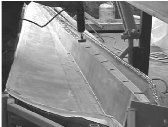
Figure 2.18 Blade Skin and Shear Web Preparation for Bonding
