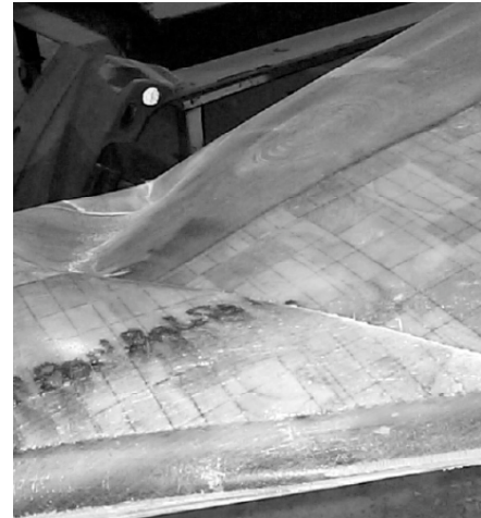
Figure 2.26 Static Failure Moment on 11 March 2002 Test
