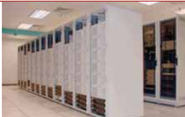
Figure 2.1-8. A PC-based visualization cluster. Cost-effective technologies are needed to enable highperformance visualization at levels well beyond today's traditional, high-end systems.
