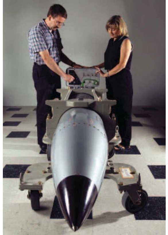
A B61-4 trainer using an aircraft monitor and control package that simulates the electronic control system of several types of military aircraft.
