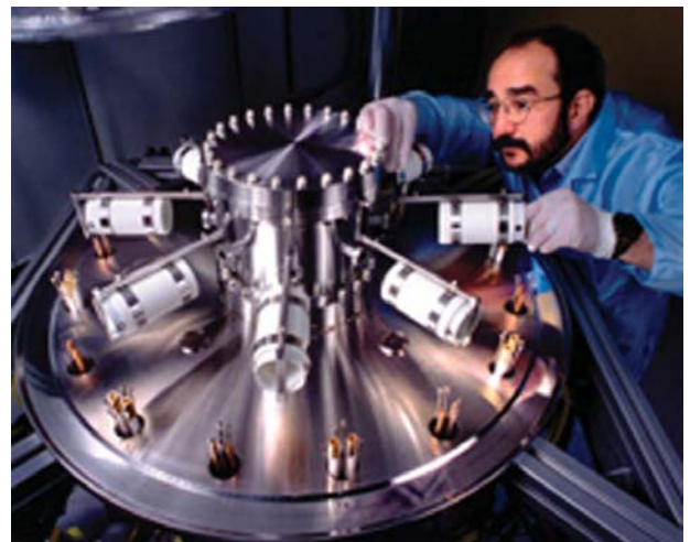
Adjustments being made at a high vacuum neutron tube bake station at the neutron generator facility.
