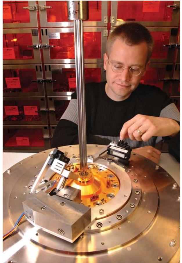
A Sandia National Laboratories researcher demonstrates the setup he and his team created to peer into the center of Sandia's Z machine at the moment of firing. The crystal under his finger is attached to portions of a Z target configuration.
