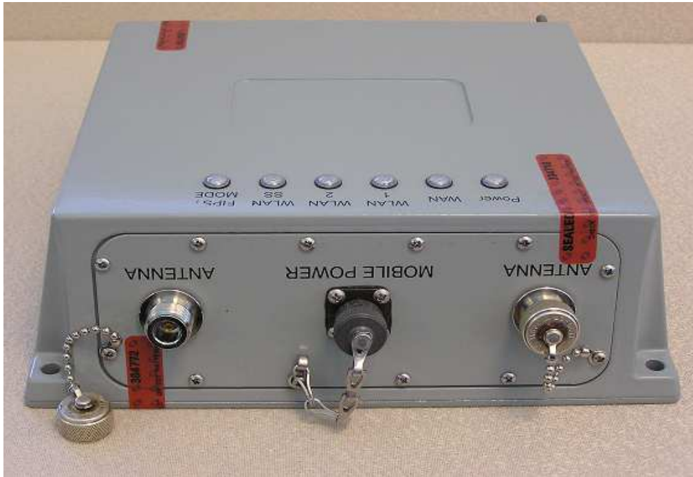
Figure 3. 3e-527A3MP Antenna Panel
