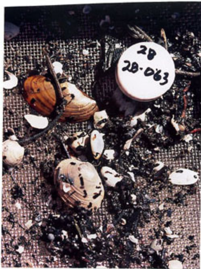
Plate 26. Typical infaunal sample from Prince William Sound, Alaska. Field samples are pre-processed (sieved), preserved, then completely sorted and identifies in the laboratory (Photo by A. Mearns, NOAA)
