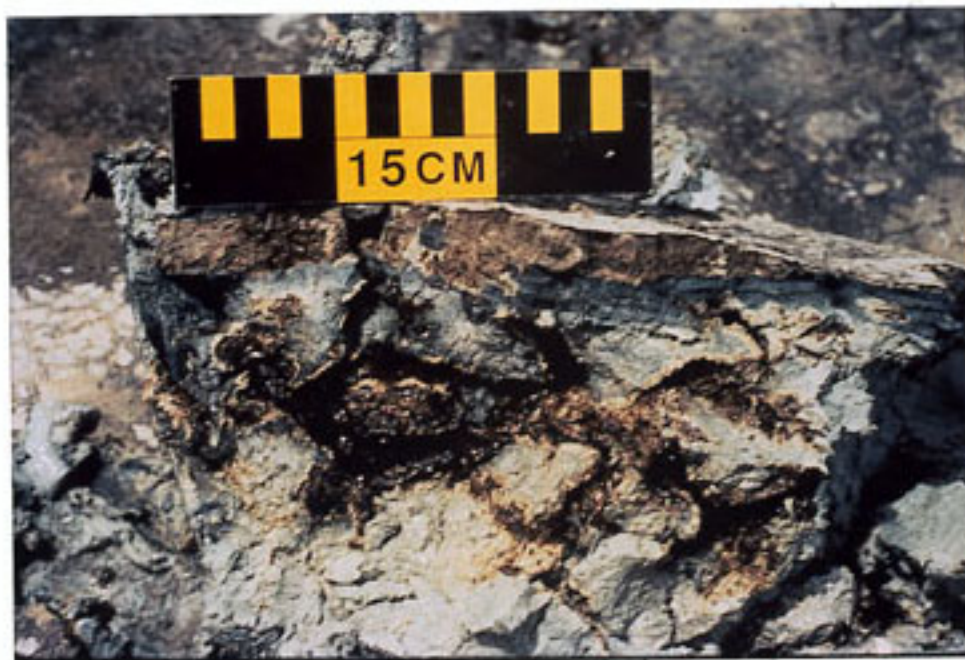
Plate 2B. February 1992 cross-section of surface sediments from intertidal mud flat in Saudi Arabian coastal zone following the 1991 Gulf War, showing penetration of crude oil via marsh crab burrows (Photo by M. Hayes, Research Planning, Inc.)
