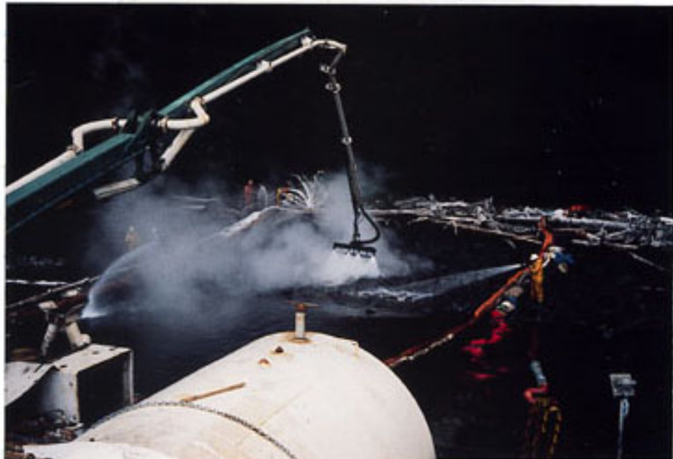
Plates 5 and 6. Two views of the "Omni-Boom" system used for high-pressure, hot-water shoreline cleanup during the Exxon Valdez spill (NOAA/HAZMAT photo).
