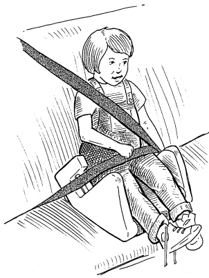
Belt positioning booster must be used with a lap and shoulder belt
