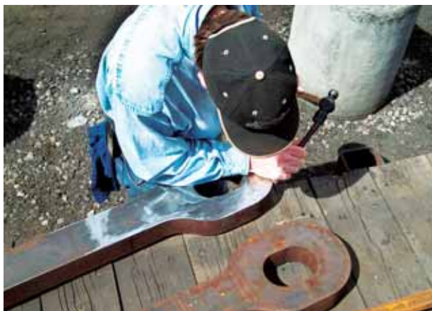
COLD CHISEL — A Cumbres & Toltec railroad worker hammers away on this massive locomotive driving rod to get a few tiny scraps of metal for Sandia to test.
