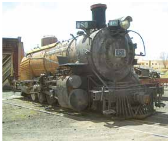
WRAPPER PLATE — Without the engine cab, the large plate surrounding this steam locomotive's boiler is revealed. This was one of several key components sampled by Sandia to help keep repairs on
