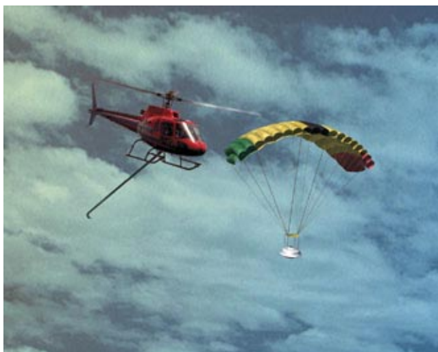
Helicopter equipped with retrieval equipment practicing a snag of the Genesis Sample Return Capsule.
