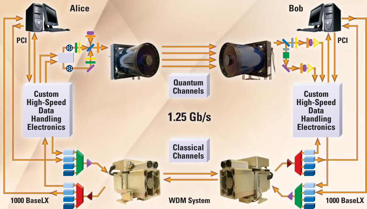
Quantum Key Distribution with 1.25 Gbs Clock Synchronization Demonstrated
