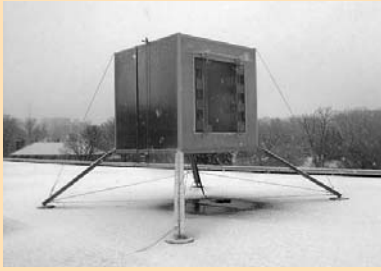
A prototype of the original "active building envelope" system on the roof of Rensselaer's Student Union building. Credit: S. Van Dessel
