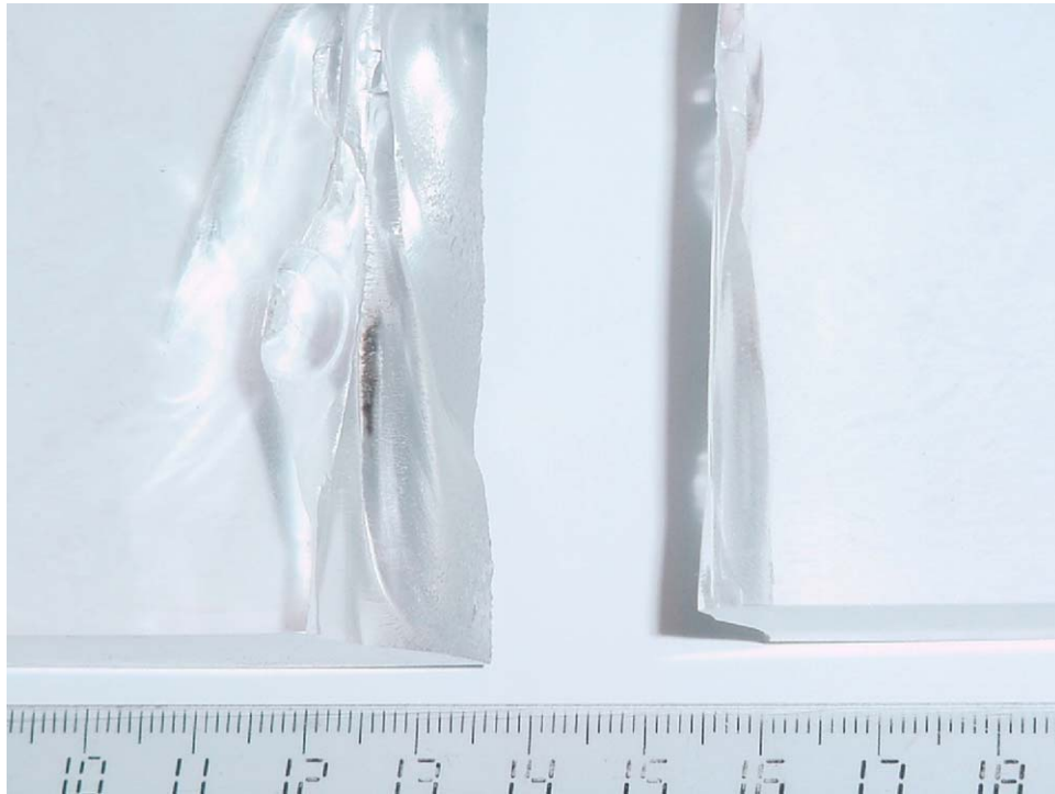
Figure P-40. Closeup view of destroyed section of the acrylic insulator (900 J).
