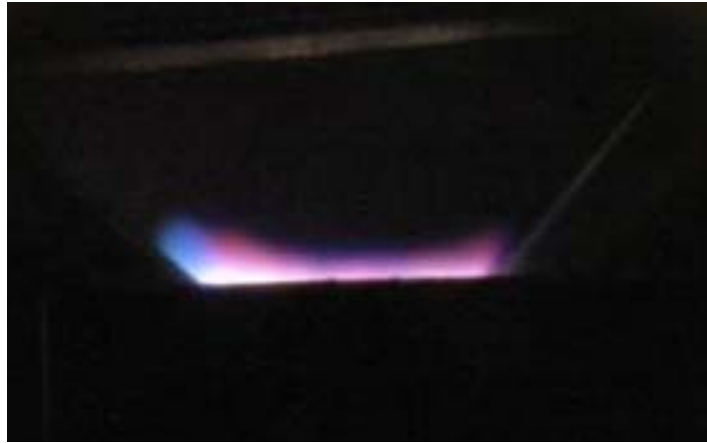
Figure Q-33. Time-integrated image of surface flashover of a polycarbonate surface in SF 6 at 10 torr. Charged electrode is on the left.
