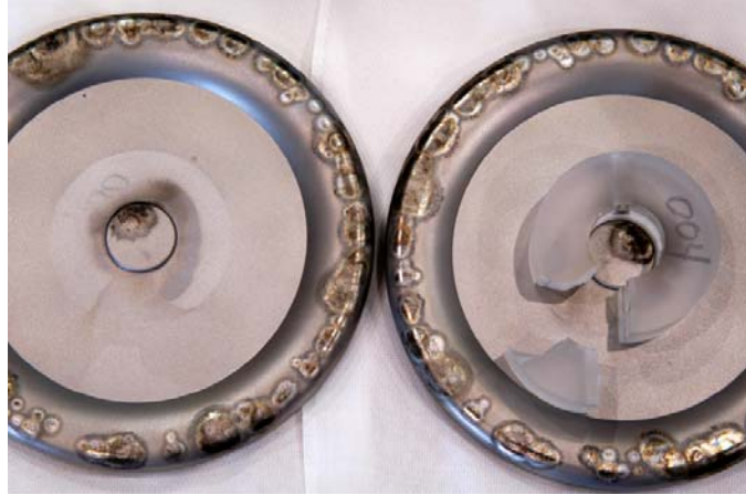
Shots 1327 – 1371: No housing flashed. Trigger plate bowed.
