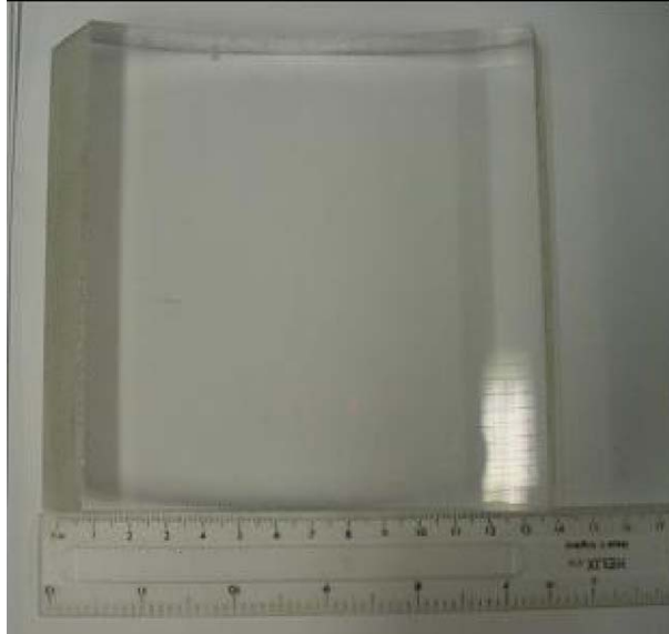
Figure P-38. The section of acrylic dielectric before high-energy tests.
