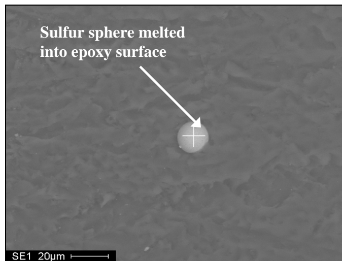
Figure 49. Scanning electron microscope image from dielectric material 826/D400/KF-865 used for X-ray spectroscopy analysis (1 atm SF 6 , 30 µC).
