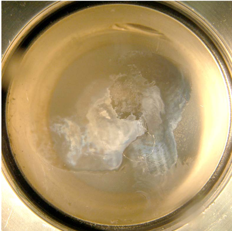
Figure D-31. The STB final optic pulled on 09-27-2006 after 93 shots. Optic shows features of HF etching, metal deposition and laser-generated UV photo-chemistry.
