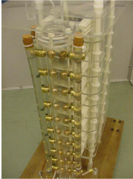
Figure P-13. Picture of the 10-stage Marx generator.
