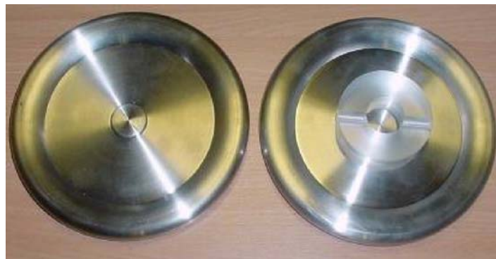
Figure P-14. Symmetrical toroidal electrodes received from SNL.
