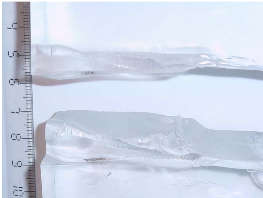
Figure P-41. Closeup view of destroyed section of the acrylic insulator (900 J).
