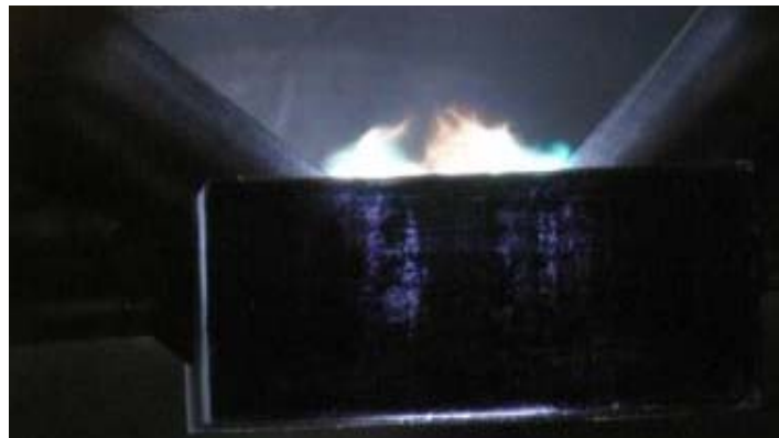
Figure Q-34. Time-integrated image of surface flashover of a Lexan surface in SF 6 at 500 torr.
