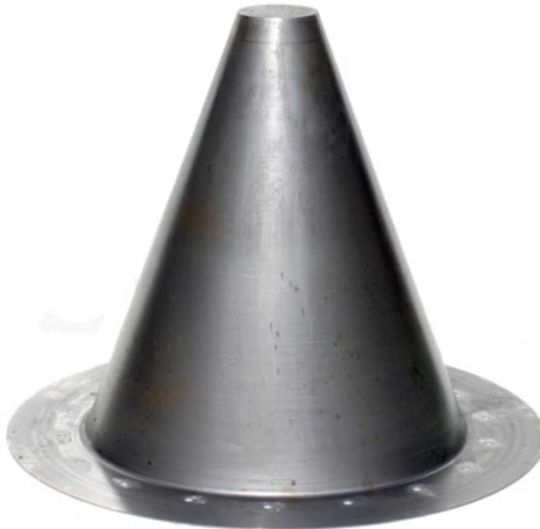
Figure 2.54. TMS Cone, showing weld and surface quality.
