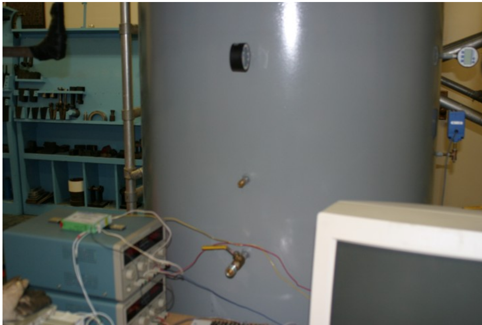
Figure 2.57. Digital pressure gage, pop-off valve, and ball valve with for air inlet.
