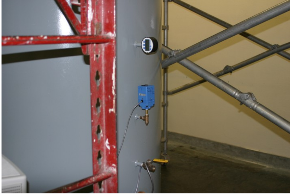
Figure 2.58. Digital pressure gage, pressure transducer, and ball valve with for air outlet/venting.
