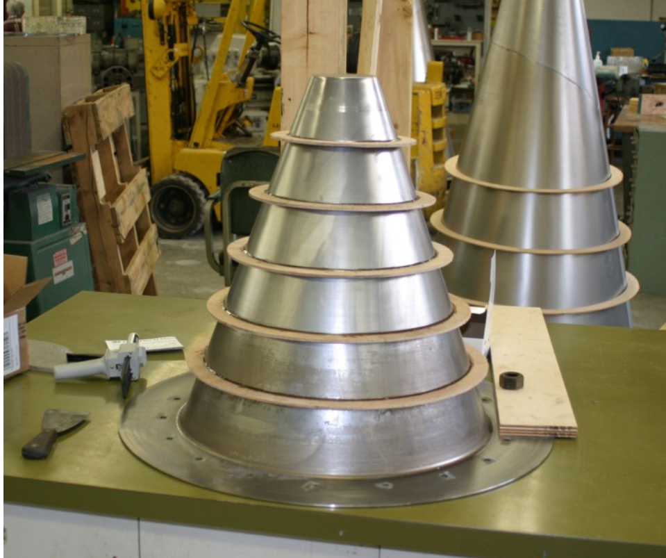
Figure 2.60. Stiffening rings mounted to cone.
