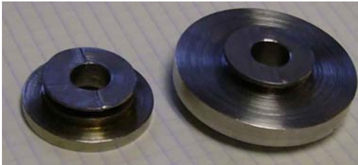
Figure 2.29. Photos of expendable electrodes, left - anode, right cathode. The central hole diameter is 10 mm, the square size on paper is 5 mm. The left half of the studied surfaces (24 mm diameter) of each electrode is covered with lead.
