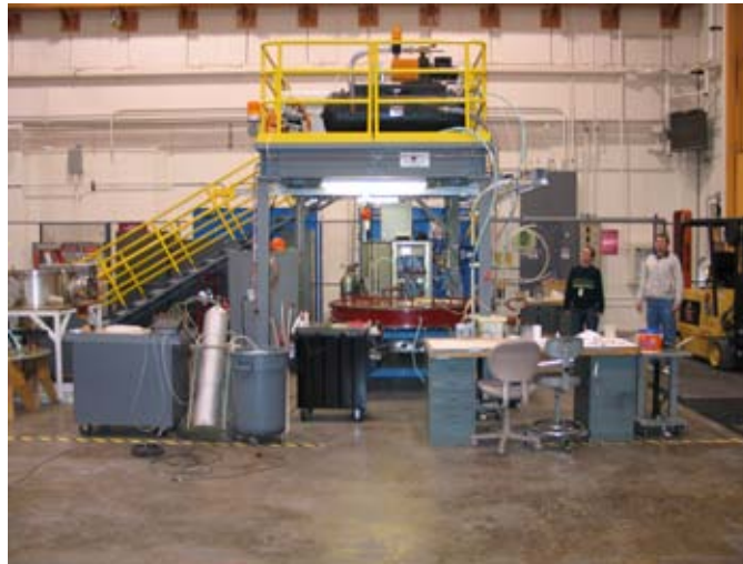
Figure 3.1. High Current LTD Laboratory at Sandia with the 500-kA LTD cavity shown at the center (red color).
