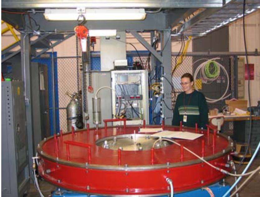
Figure 3.2. Close up view of the LTD cavity, the various cable and air hoses connecting to the cavity are visible.
