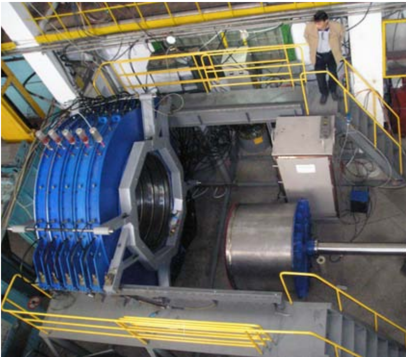
Figure 3.9. Top view of the LTD voltage adder with the cathode electrode removed and located in front of the LTD anode vacuum cylinder.
