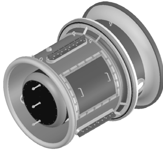
Figure 84. The physical layout of the PFL with a view of the water spark gap switch shown.
