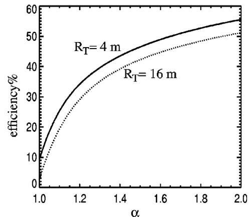
FIG. 10. The efficiency is plotted as a function of  $\alpha$  for two values of the transmission line outer radius.
