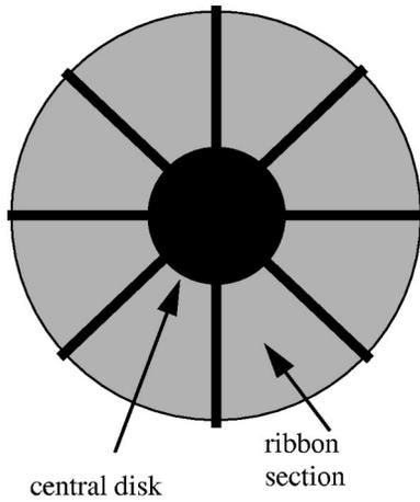
FIG. 11. A schematic of a disk electrode composed of triangular ribbon sections.
