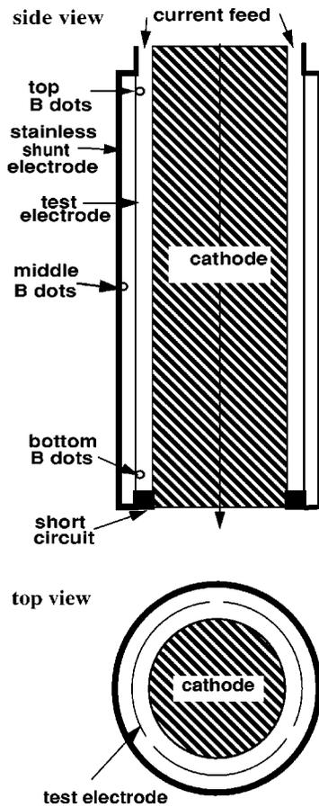
FIG. 2. A schematic of the experimental design.
