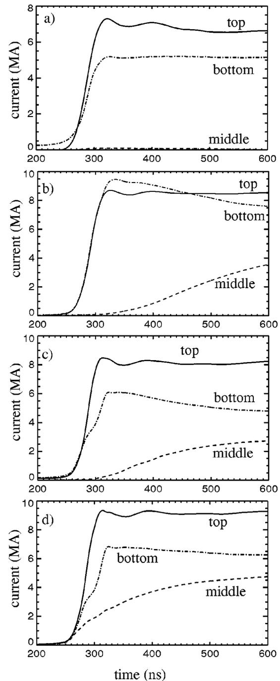
FIG. 3. The currents plotted as a function of time for (a) 250  $\mu\text{m}$  carbon steel, (b) 100  $\mu\text{m}$  carbon steel, (c) 50  $\mu\text{m}$  carbon steel, and (d) 20  $\mu\text{m}$  of mylar.
