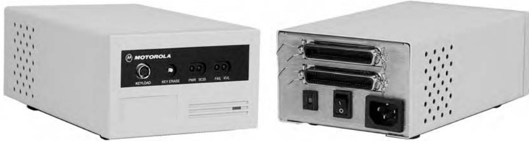
Figure 1: HW kit T7289A. The Crypto Boundary includes the entire encryption module and housing. The module contains 3 connectors: SCSI (Data, Control, Status, and OTAR Key data) connector, KVL (Key Data, Control, and Status) connector, and Power Connector. The module also contains a Key Erase button (equivalent to tamper) and 4 status LEDs.
