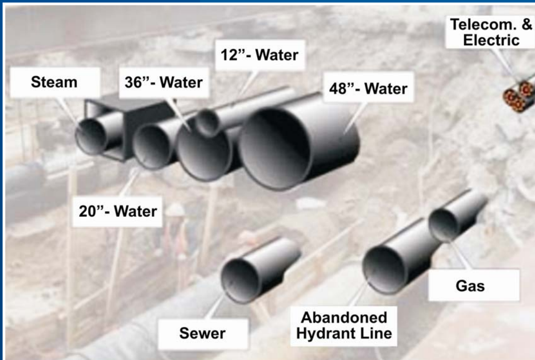
Cross Section of NYC Street Showing Utilities
