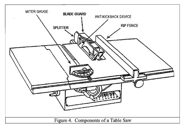
A typical antikickback device consists of pawls, which have teeth that are designed to grab the work piece if it begins to reverse and prevent it from being thrown back towards the operator. The antikickback pawls are also attached to the splitter (see Figure 4).
