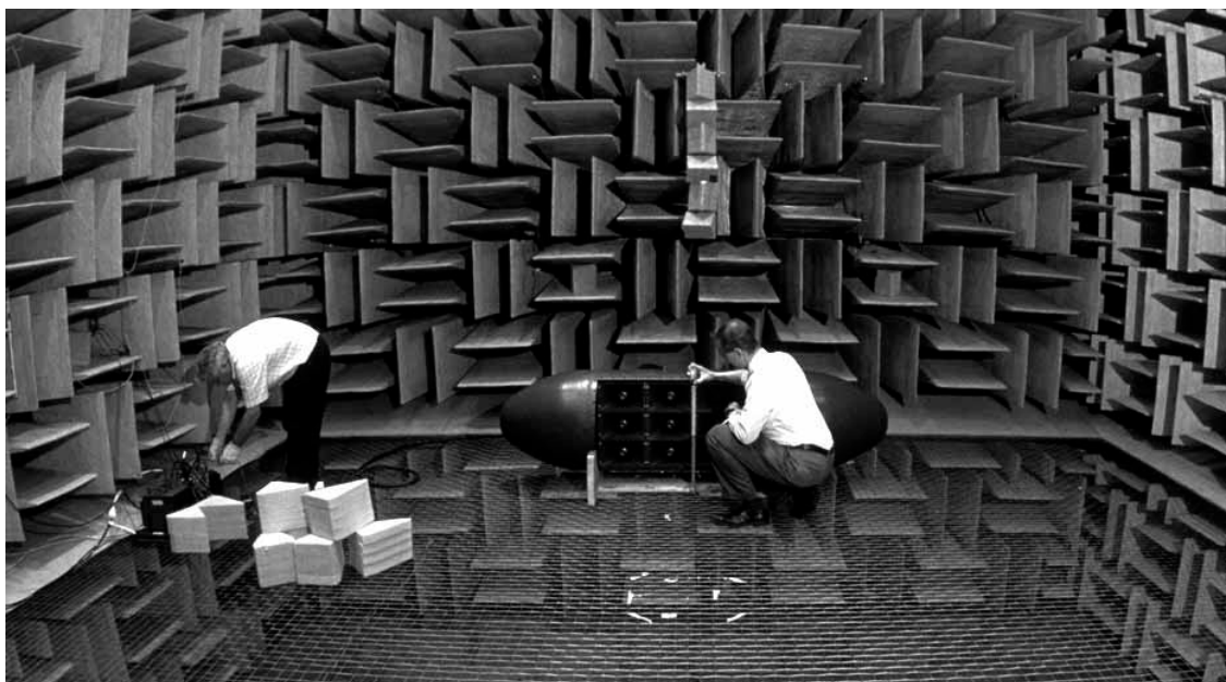
Army helicopter loudspeaker unit setup for testing in the acoustic anechoic chamber research facility
