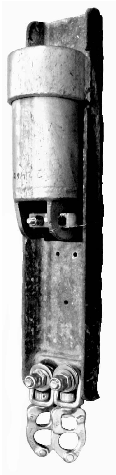
Figure 3. Photo of the bottom contact sensor and its attachment configuration to the ground gear used during the 2004 BSS survey.
