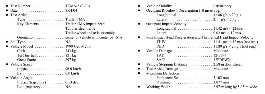
Figure 21. Summary of Test Results and Sequential Photographs, Test TTMA-3
