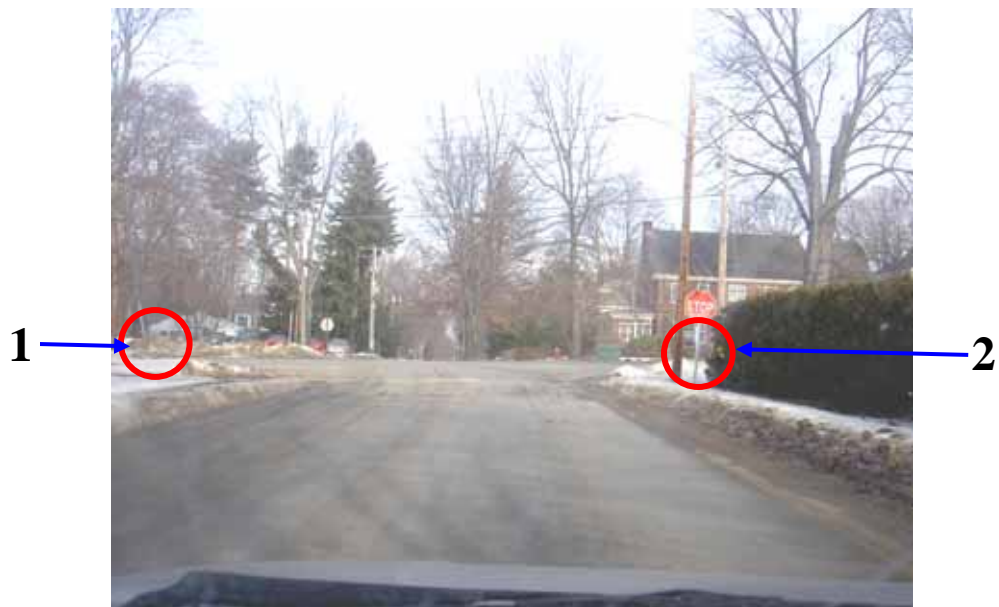
Figure 6e: (1) Cross Traffic From Left; (2) Area From Which Hidden Pedestrian May Emerge
