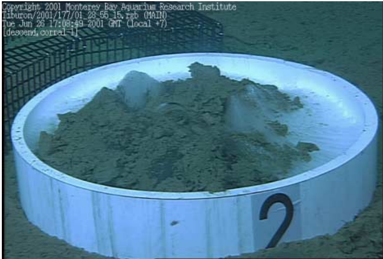
Figure 1. Image of a mass of CO 2 hydrate formed on the sea floor at 3,600m depth by penetration of liquid CO 2 into the sediment followed by hydrate nucleation (Brewer et al., 2001).
