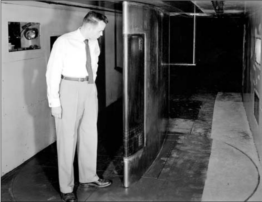
Figure 4-5. Researcher Dean Bowden inspects pneumatic de-icer on NACA 0011 airfoil model in IRT, 1948. (NACA C-35792)
