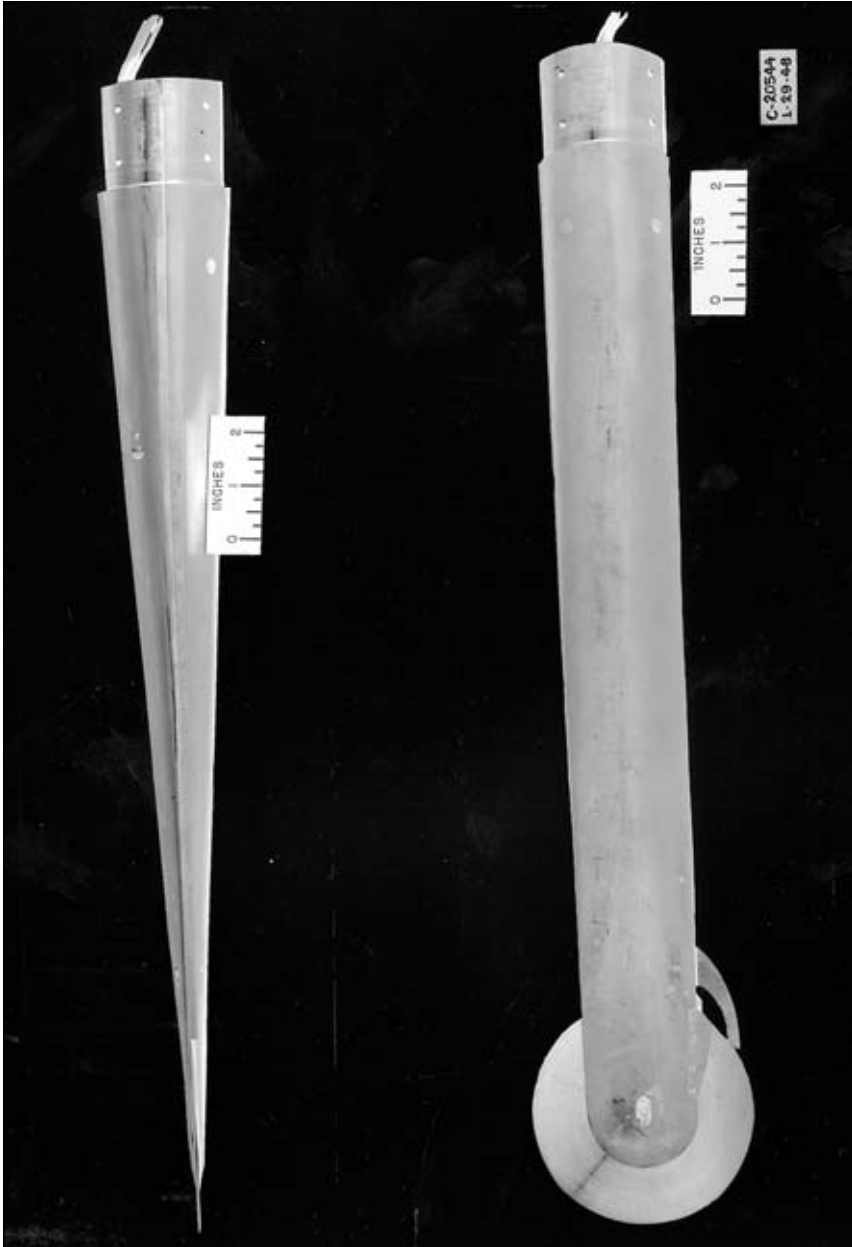
Figure 3-11. Rotating disk icing rate meter, 1948. (NACA C-20544)
