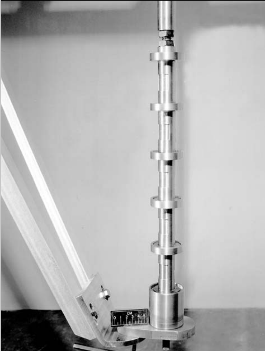
Figure 5-9. Ice-phobic test rig designed by Raymond Sotos, 1980. (NASA C-80-685)
