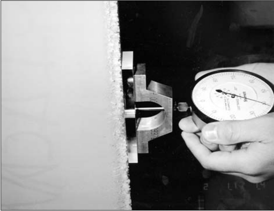
Figure 6-13. Measuring leading-edge thickness, 1990. (NASA C-1990-12947)
