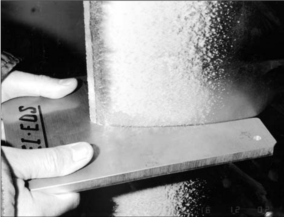
Figure 6-12. Metal template melting ice accretion for profile check, 1990. (NASA C-1990-13574)
