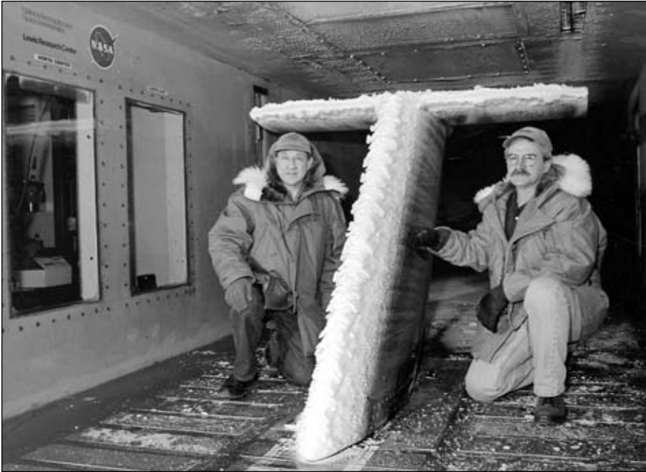
Figure 8–13. Bell Augusta 609 tilt rotor empennage during icing tests, 1999: (L/R) technicians Tom Lawrence and Michael Lupton. (NASA C-99-204)
