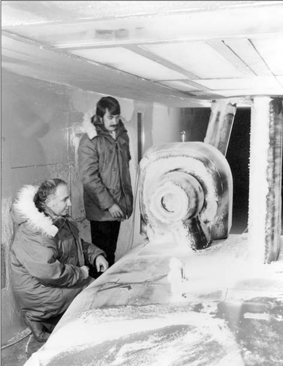
Figure 5-8. Raymond Sotos (kneeling) and David Justavick with Hughes A-64 inlet after icing test, 1980. (NASA C-80-1729)
