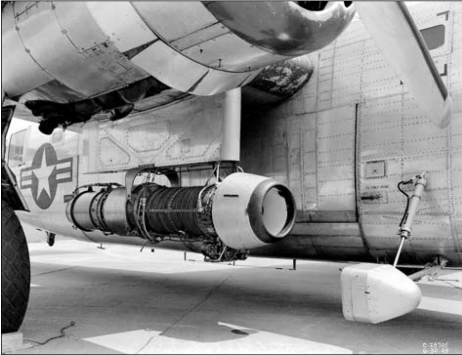
Figure 4-2. Westinghouse 24C-2 turbojet engine under wing of B-24, 1949. (NACA C-23705)
