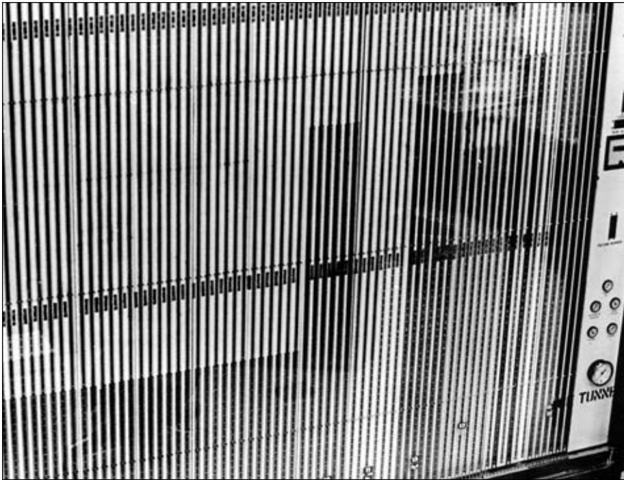
Figure 4-11. Bank of manometer tubes used to record pressure on a model in the IRT test section. (NACA C-161503-5)
