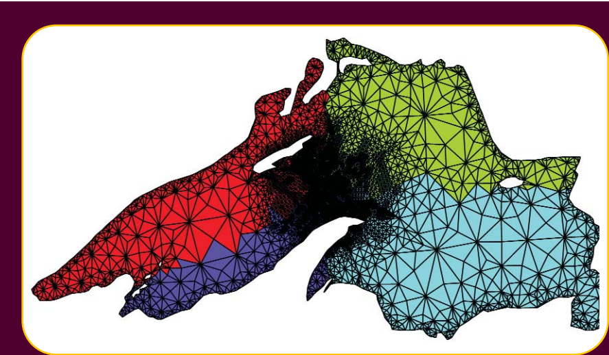
ITL's PHAML software for the parallel adaptive solution of partial differential equations has recently been extended to deal with complicated spatial domains. This image shows an adaptive grid computed by PHAML for Lake Superior.
