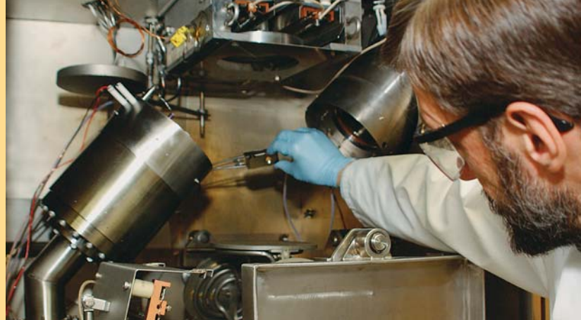
John Snyder adjusts the secondary ion-beam gun that is used in etching the surface of thin films created in the deposition system.
