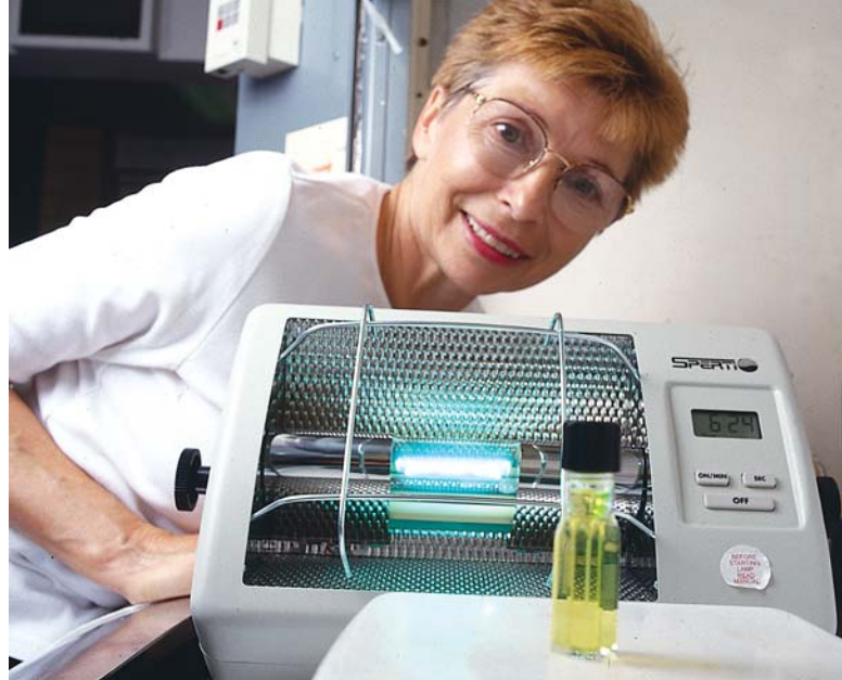
Andreja Bakac observes photolysis (chemical decomposition induced by light) in a reaction solution as part of a catalysis experiment.
