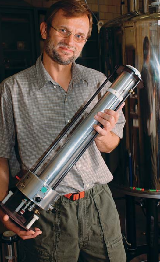
Marek Pruski displays one of the probes used with the NMR equipment in his laboratory. The turbine in the probe spins the sample at almost two million rpms to overcome the broadening of spectral lines.
