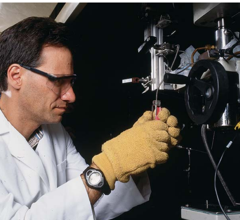
Brent Shanks draws a sample of the conversion product from a batch reactor. This sample will be analyzed for yield of the desired dibasic acid product.
