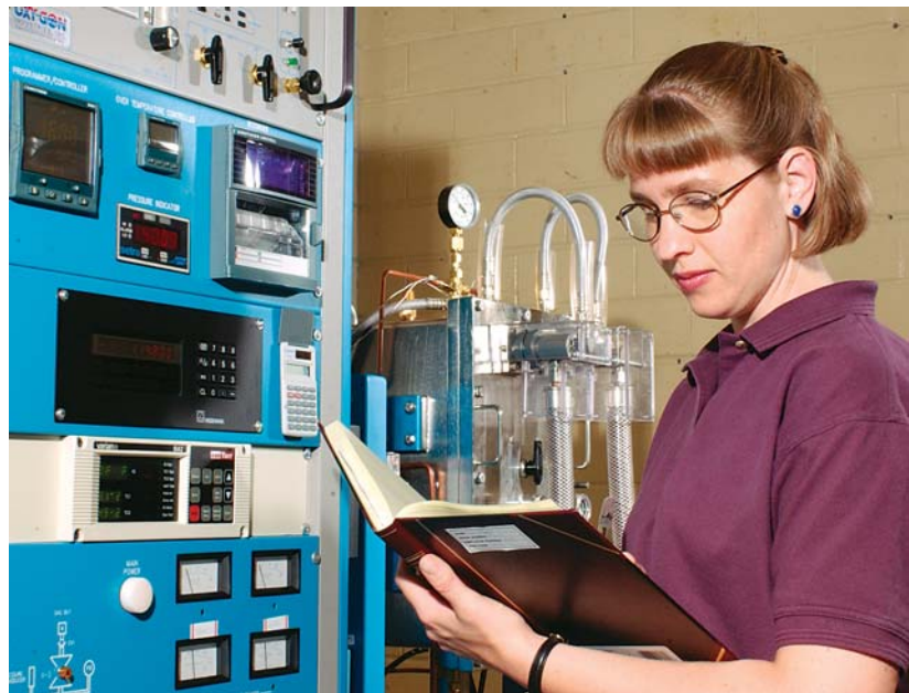
Ames Laboratory assistant scientist Amy Ross checks the status of a crystal sample being grown in the High-temperature Bridgman furnace, one of many specialized pieces of equipment found in the Materials Preparation Center.
