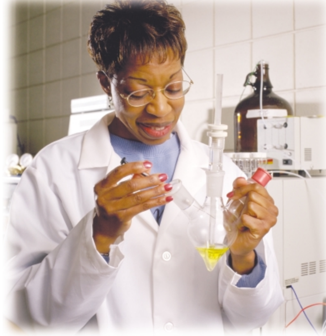
Sheares removes a sample from a polymerization mixture to isolate it for characterization.
