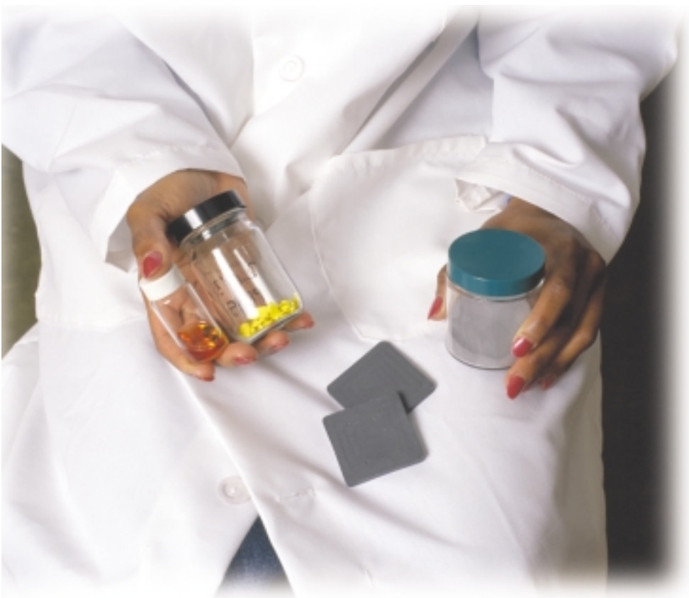
In jars, from left: a polymer solution, isolated polymer and pure quasicrystal filler are the ingredients for a new composite that is highly resistant to wear, nonabrasive and easy to process.
