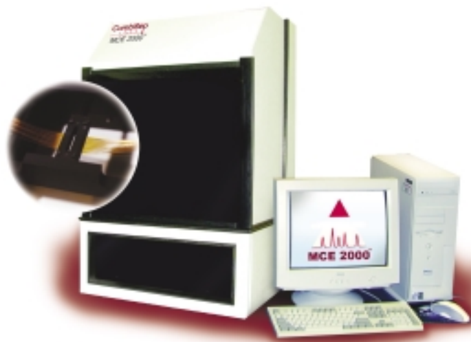
The MCE 2000 is a multiplexed, absorbance-based capillary electrophoresis system made by CombiSep, Inc. The system can perform 96 separations simultaneously through its array of 96 capillary tubes (inset).
