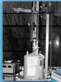
◀ Magnetic refrigeration was proven possible using a gadolinium-silicon-germanium alloy developed by Karl Gschneidner and Vitalij Pecharsky.
