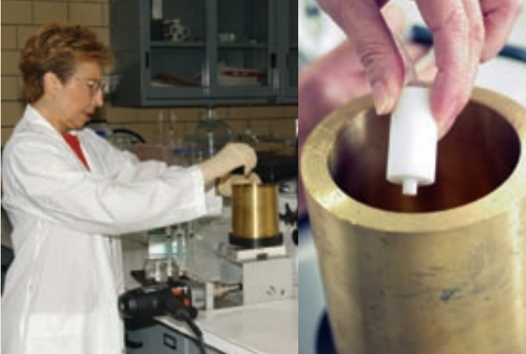
(left) Preserving a life: Andreja Bakac demonstrates the device that allows her and Oleg Pestovsky to generate and freeze iron(IV) in less than a second.
