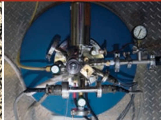
The tunnel diode resonator allows experimental sensitivity far exceeding commercial setups for studying the properties of superconducting materials.
