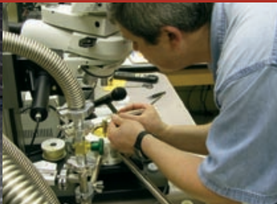
Ruslan Prozorov prepares a sample for low-temperature magneto-optics study. He applies his own unique measurement techniques to analyze the relationship between the patterns created in the presence of a magnetic field and the macroscopic magnetic properties of the material.
