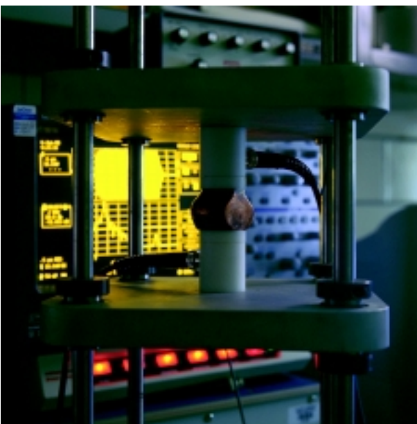
As short pulses are shot into the copper crystal, the frequencies generated by the microstructure are shown on the oscilloscope behind the sample holder.
