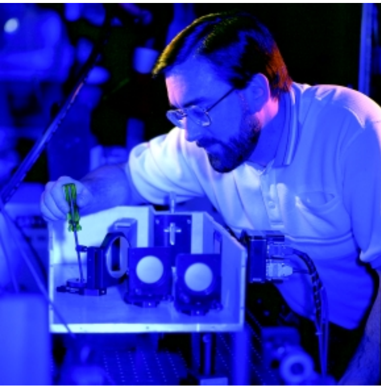
Ames Lab assistant chemist Dan Zamzow makes adjustments to the echelle spectrometer of the mercury CEM.
