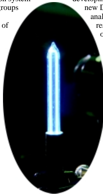
An ordinary pen lamp is a key piece of equipment in the mercury CEM.
