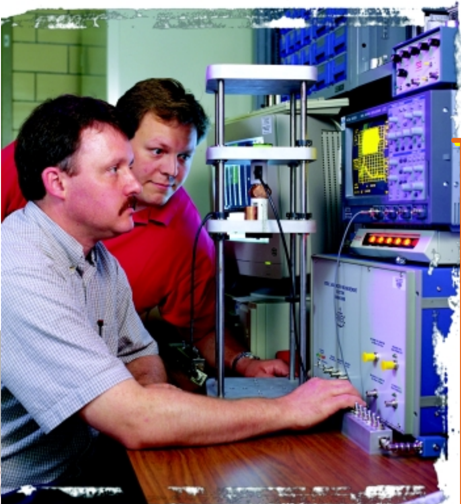
Dan Barnard (foreground) and Jim Foley use acoustic harmonic generation techniques on a single crystal of copper that sits in the middle of the three-tiered apparatus.
