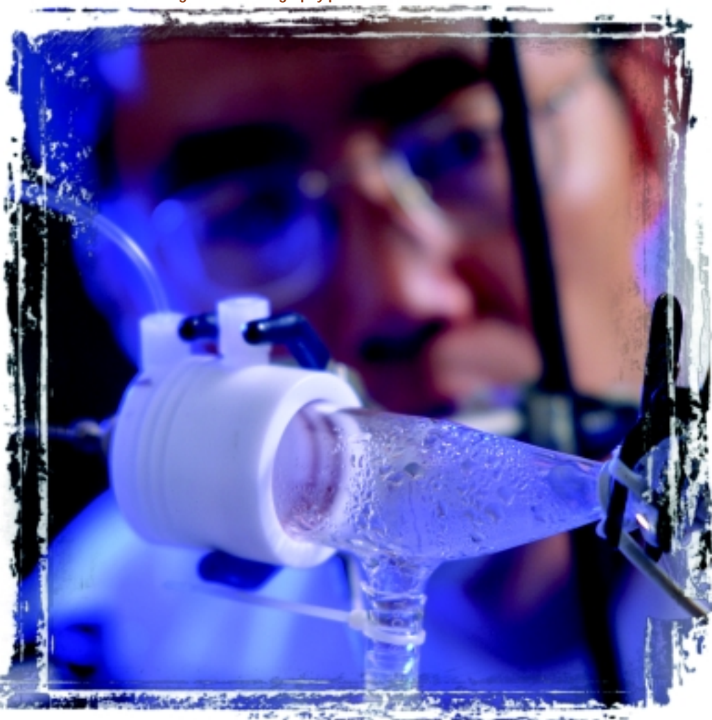
Jin Wang observes the fine droplets of mist created when a sample is injected into the nebulizer following the chromatography process.
