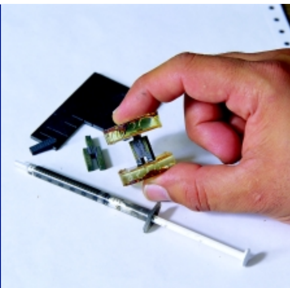
The small platforms consist of three pieces of silicon carbide composites that were glued together, with plastic discs at the ends. Seven such platforms supported the weight of the three researchers in the photo at left.
