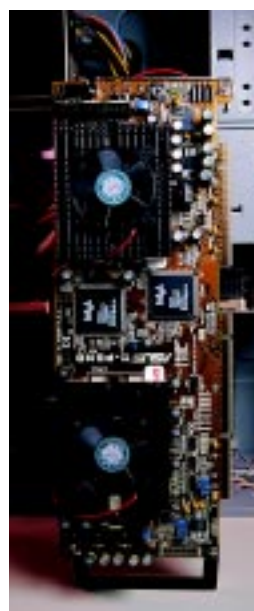
Each personal computer in the SCL’s 64-node cluster contains two central processing units, making a powerful system of 128 processors.
