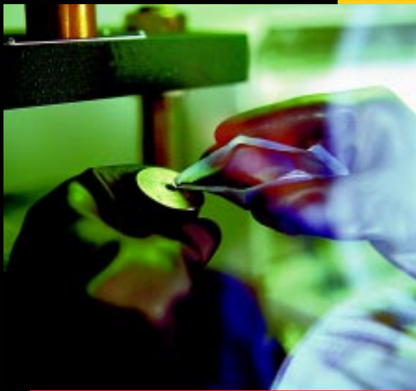
To avoid contamination, pellets of the silicide material are studied in the oxygen-free atmosphere of a glove box.
