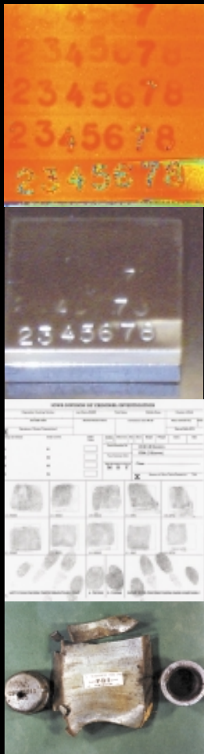
Among the current forensic projects at Ames Lab and IPRT are restoring serial numbers (top photo) that have been removed from hard metals (second photo); better fingerprint detection methods (third photo); and analyzing bomb-blast fragments (fourth photo).
