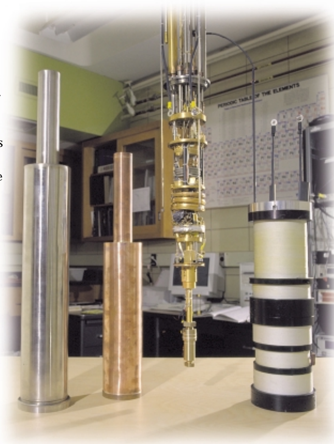
Essential components of Ames Lab's new combined extremes facility are (left to right): high-vacuum can, heat shield, dilution cryostat with attached high-pressure cell, and the superconducting solenoid.
