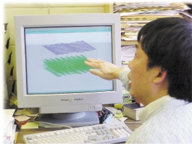
Using an atomic simulation he developed, Cai-Zhuang Wang demonstrates how carbon atoms (purple circles) are peeled from the diamond surface in a layer-by-layer fashion when subjected to femtosecond laser pulses.
