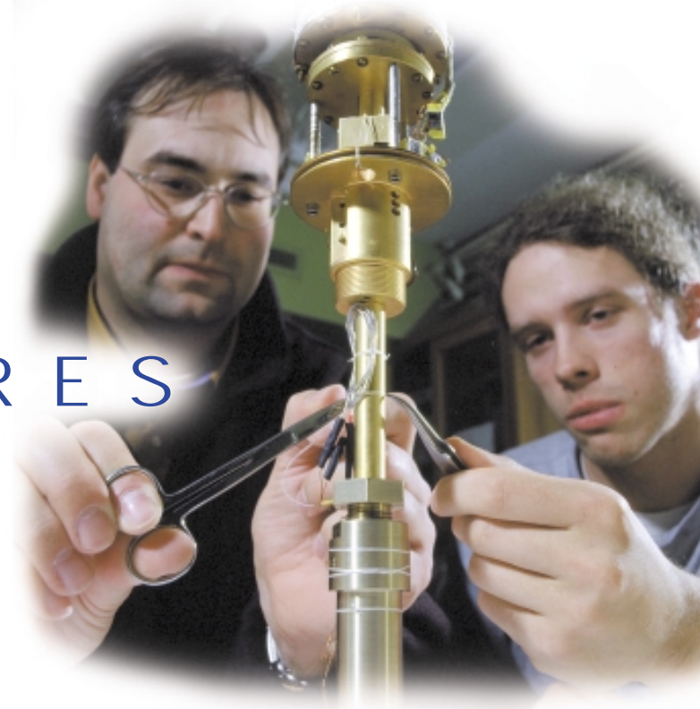
Robert Modler (left) and Andrew Thomas prepare an experiment to investigate materials under simultaneous extreme conditions of very low temperature, high pressure and high magnetic field.
