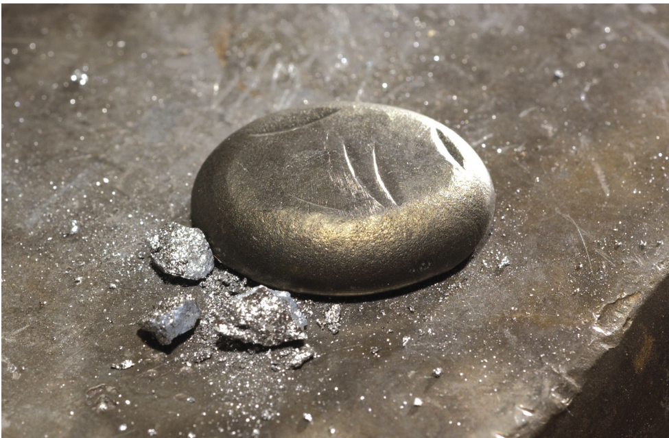
The yttrium-silver button shows dents and deformation from repeated hammer blows. The gadolinium-silicon-germanium material was shattered with a light tap from the hammer.
