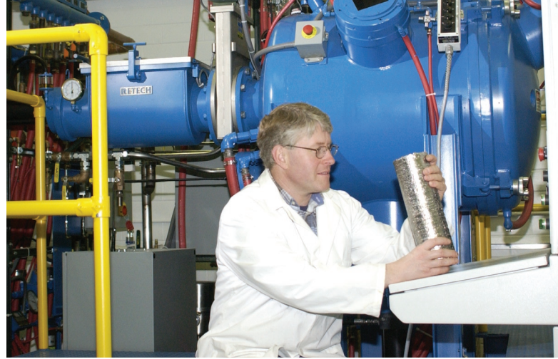
Research technician Arne Swanson holds an ingot of material that was consolidated in the bright blue Retech 150 plasma furnace, shown behind him in the Materials Preparation Center.
