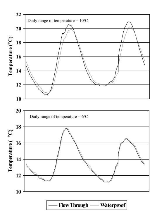
Figure 1. Comparison of 2 days of recorded temperatures for data loggers placed in two streams. Each stream had a data logger placed in a flow through housing and a data logger placed in a sealed (waterproof) housing.
