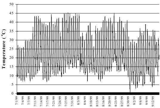
Figure 7. Example of temperature measurements from a site that was dewatered during the sampling period. Note the extreme (>30 °C) daily fluctuation in temperature, and extraordinarily warm (>40 °C) temperatures.
