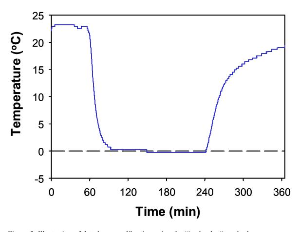
Figure 3. Illustration of data logger calibration using the "ice bucket" method.
