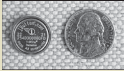
Figure 5.25 – Temperature recording technology has become smaller and very inexpensive. The iButton® shown next to the nickel can record more than a year of temperature data.
