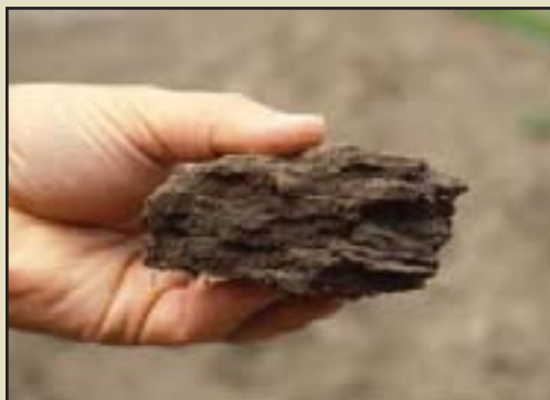
Figure 5.14 – Compacted soils are created by heavy equipment operating over soil. The large pore spaces are compressed and the soils often form a platy structure as shown in this photograph.
