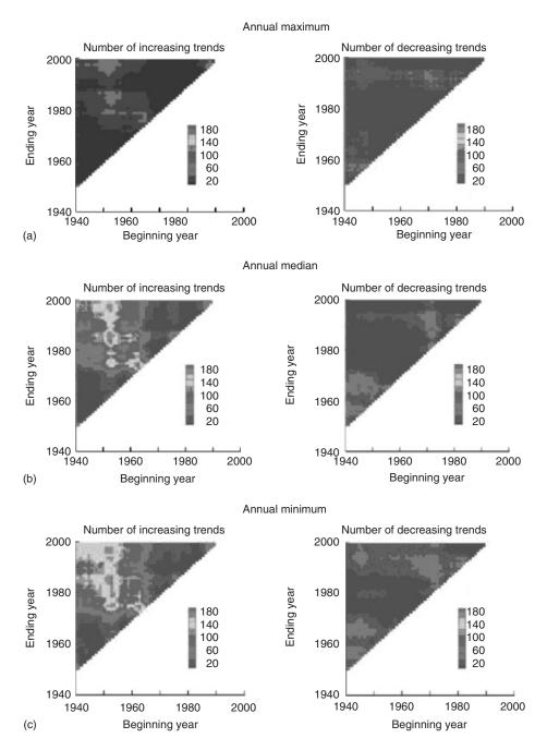
**Figure 3** Number of sites with significant ( $p \le 0.05$ ) increasing and decreasing trends in (a) annual maximum, (b) median, and (c) minimum daily streamflow for various periods at least 10 years in length, and for 400 stations in the United States during 1941–1999 (Reproduced fromMcCabe and Wolock, (2002 ) by permission of American Geophysical Union (AGU)). A color version of this image is available at http://www.mrw.interscience.wiley.com/ehs
