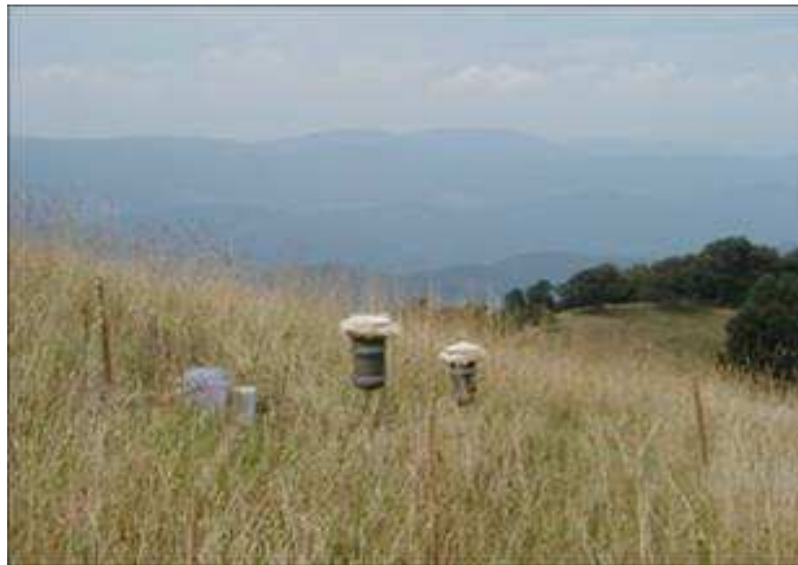
Figure 1. Recording unit, Nelson Sods, Pike Knob Preserve (TNC), Pocahontas Co., WV. Microphones, two per unit, are nestled in PVC housings covered by shag wind screens. Sounds are recorded onto an mp3 recorder with 100 GB hard drive, housed in a weather-tight access box mounted on a bucket that holds the batteries.
