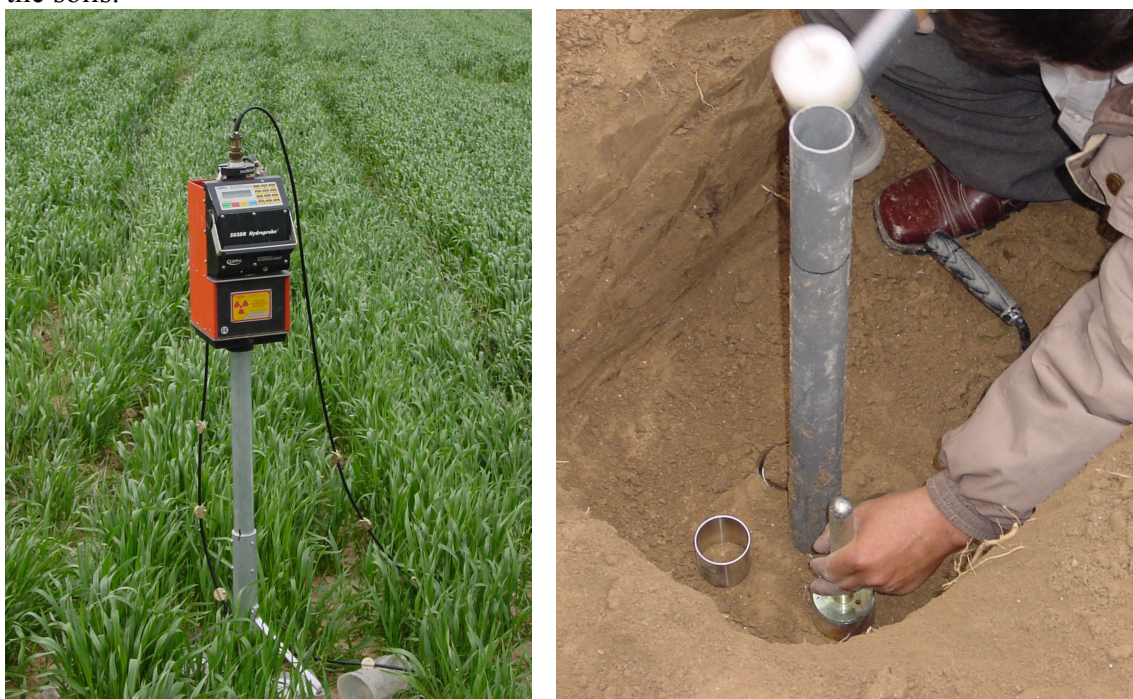
Figure 1 Left: A soil moisture neutron probe in position on a depth control stand while recording a standard count. Right: Four volumetric soil samples were taken around each access tube at each depth. Shown are the 100 cm 3 sampling cylinders.
