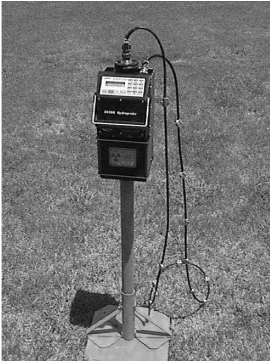
Example of CPN profiling neutron moisture meter resting on depth control stand
