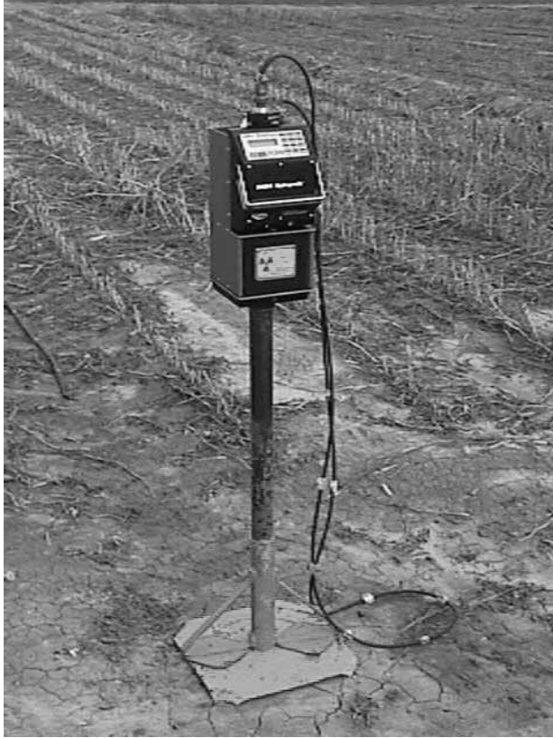
Depth control stand used to elevate a model 503 DR NMM during a standard count
