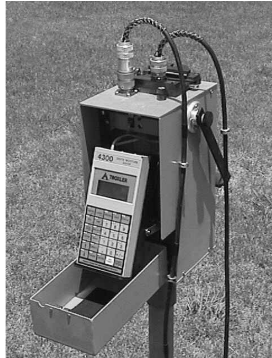
Example of Troxler profiling neutron moisture meter resting on depth control stand
