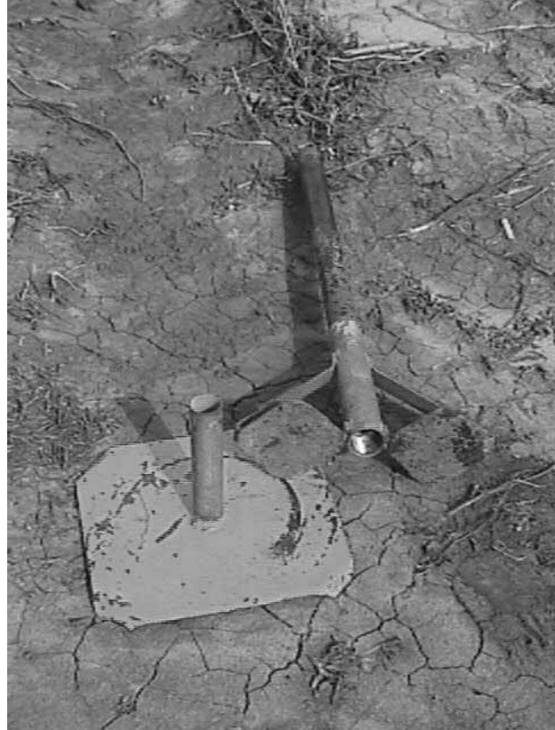
Base plate used to stabilize the depth control stand during standard counts, and the stand
