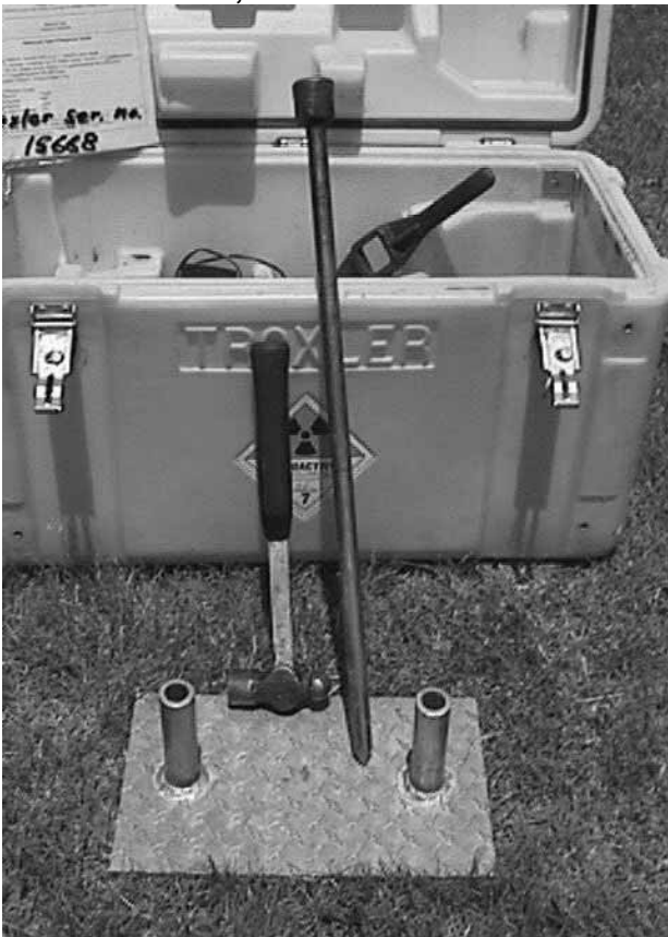
Moisture/density gauge accessories: Type A case, scraper/guide plate, drill rod, hammer, and rod removal tool
