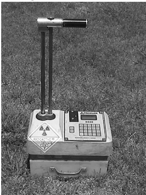
Gauge with source rod secured
