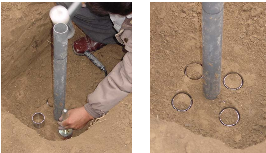
Figure 3.1.3.10-3. Sampling the NMM measurement zone with volumetric cylinders. The black mark near the top of the access tube indicates the original soil surface and is used to measure the depth of soil removal prior to sampling.
