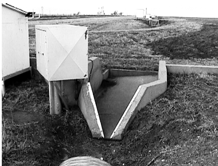
Fig. 5.38 H-flume and recorder (in white box) for measuring runoff rate from a graded bench terrace at Bushland, TX. Note dike diverting flow from uphill flume
