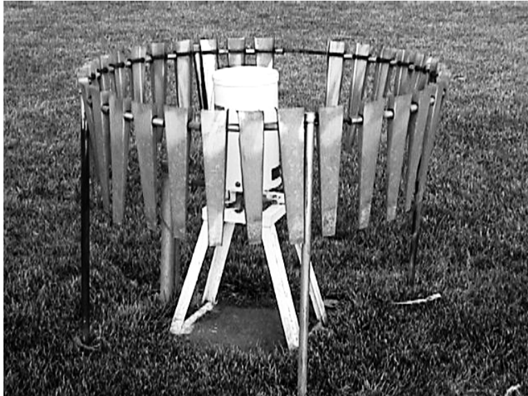
Fig. 5.39 Wind shield installed around a heated, tipping bucket rain gauge
