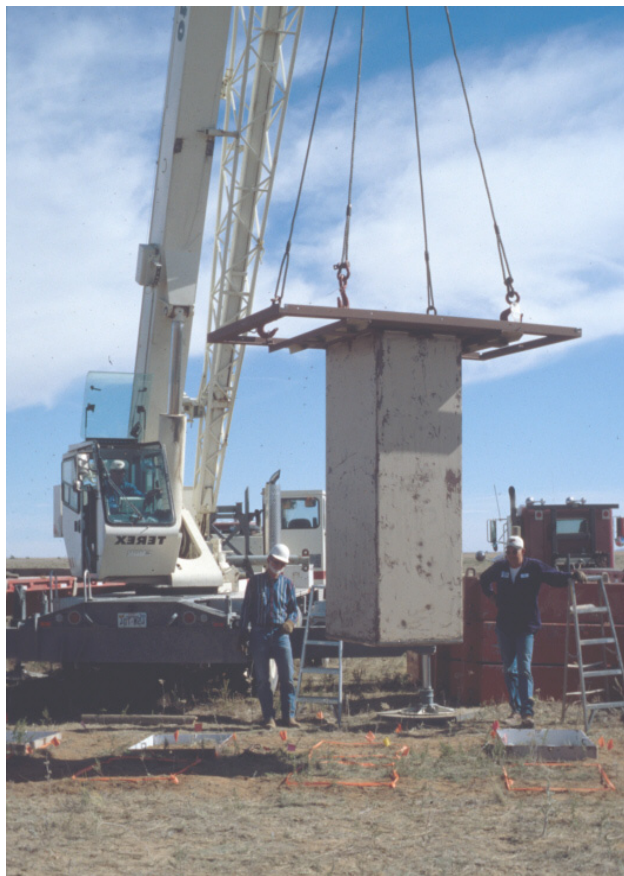
Figure 3. Lysimeter box being moved into position for collection of a Vingo soil monolith.
