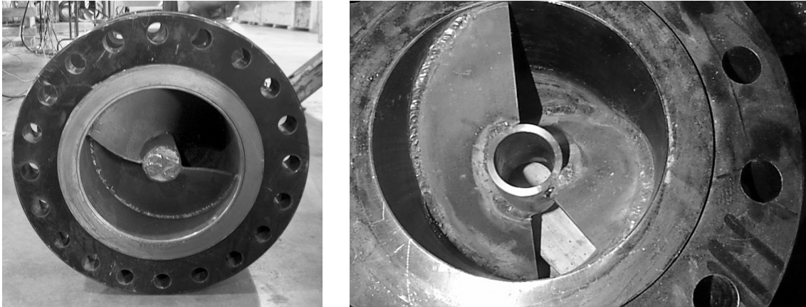
Fig. 2 – Pictures of swirling spool used during the pre-test. This device was used to introduce an axisymmetric component of swirl (i.e., and arbitrary installation effect) into the flow.
