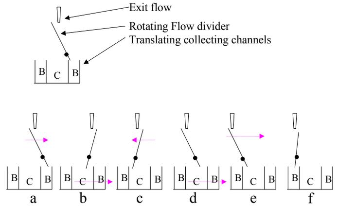
**Figure 8.** Option III – A rotating diverter valve with translating flow-directing channels.
