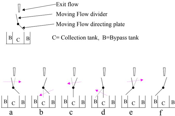
**Figure 6.** Option I – A rotating diverter valve with a rotating flow-directing device. Tanks are stationary.
