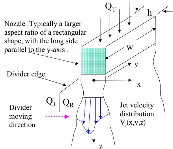
Figure 2. Liquid jet and diverter.
