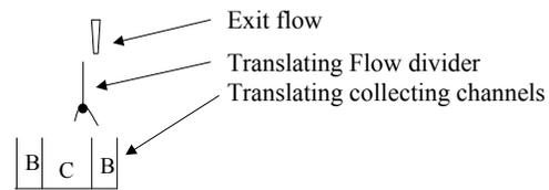
**Figure 9** Option IV – A translating diverter valve with translating flow-directing channels.
