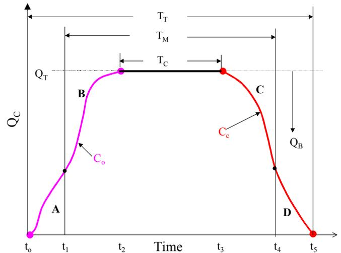
**Figure 1.** Liquid flow collected as function of time. For clarity, the constant collecting flow interval,  $T_C$ , has been compressed.
