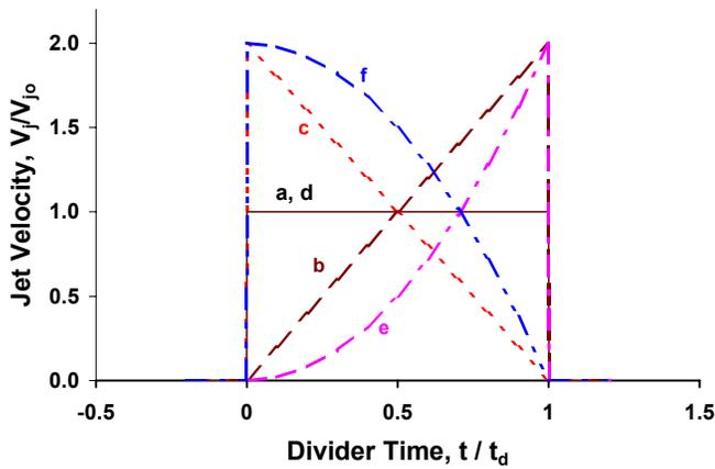
**Figure 4.** Jet velocity distribution as function of the diverter valve movement time. [Case (a) = Case (d)].
