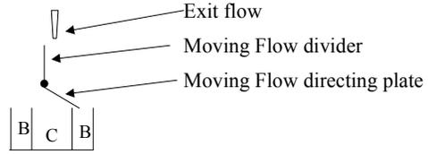
**Figure 7.** Option II – A translating diverter valve with a rotating flow-directing device. Tanks are stationary.
