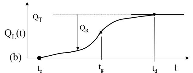
**Figure 3.** Divided flows as function of flow diverter position or time.
