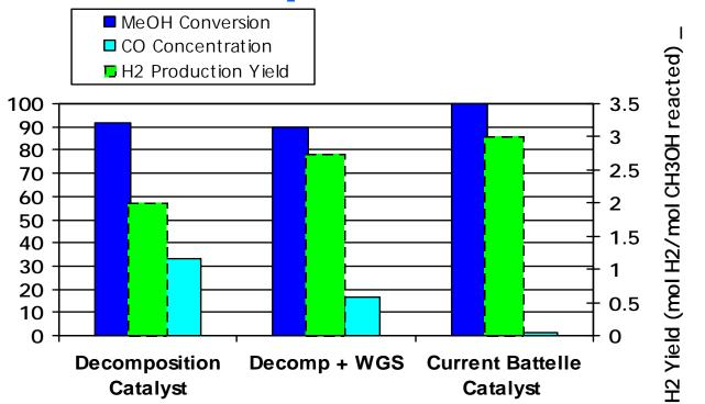
+ For methanol reforming the  $H_2$  yield is close to theoretical maximum
