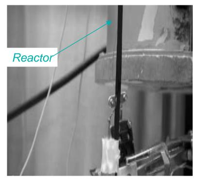
reformer volume: <5.0 mm<sup>3</sup> reformer capacity: 200 mW combustor volume: <5.0 mm<sup>3</sup> combustor capacity: 3 W National Laboratory Operated by Battelle for the
