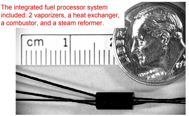
reformer volume: <5 mm<sup>3</sup> reformer capacity: 200 mW combustor volume: < 5 mm<sup>3</sup> combustor capacity: 3 W
